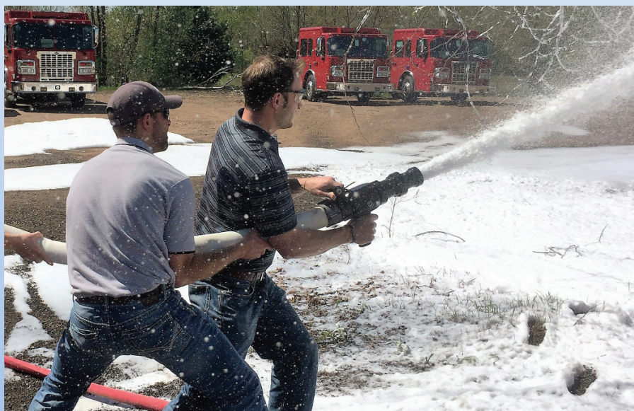
Hose handling characteristics of high-energy CAFS lines require additional training and understanding
